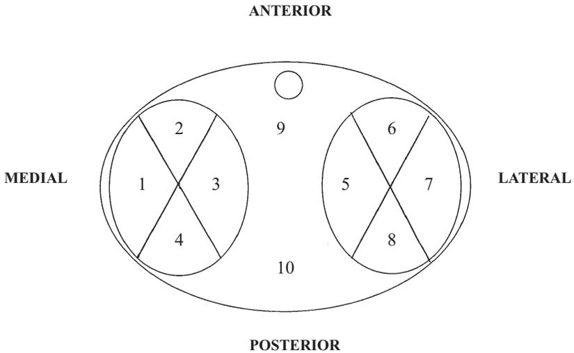
*Figure 7.8. Sections 1 to 10 of the polyethylene insert, used to locate the damage.*
