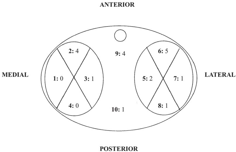
**Figure 7.20.** Number of inserts with screw impressions in the ten different sections of the tibial insert.
