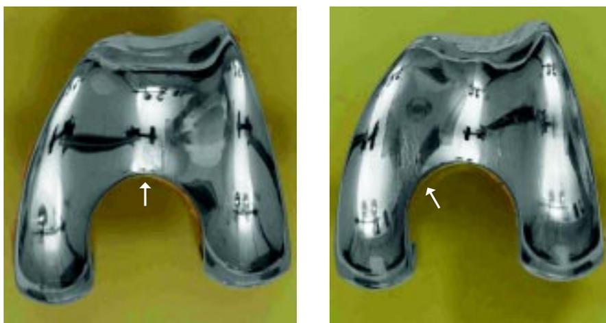
**Figure 7.21.** Marks of the screw were seen as marks of the thread of the screw in one femoral component (left) or marked scratches (right).
