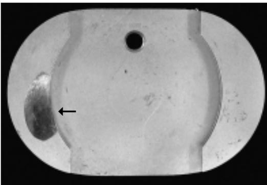
**Figure 7.24.** Damage of the metal tibial baseplate due to metal-on-metal contact.
