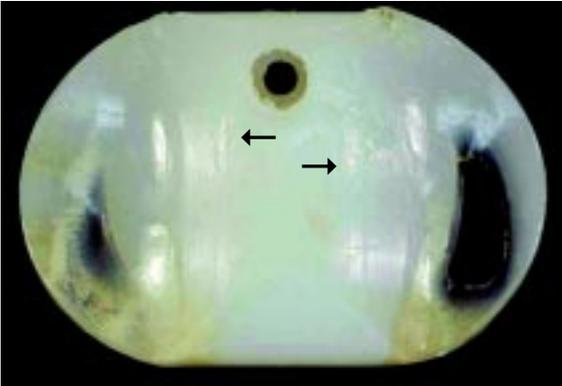
**Figure 7.2.** Scratching: indented lines generally found in an antero-posterior direction and in the areas of wear.
