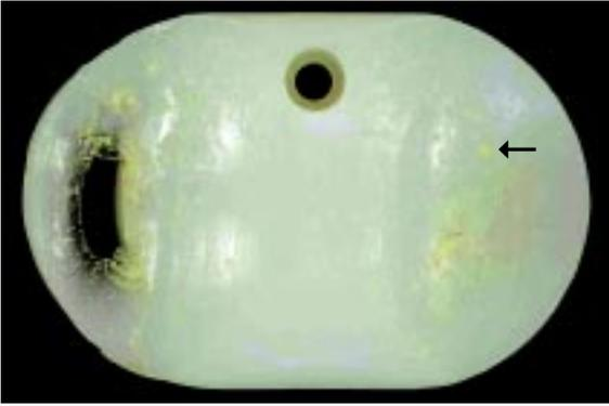
**Figure 7.7.** Bone-cement debris: embedded PMMA or bone debris, recognized by the color and/or texture difference between PMMA, bone and polyethylene.
