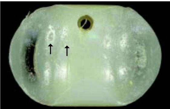
**Figure 7.3.** Pitting: depressions in the articulating surface, measuring 2-3 mm across and 1-2 mm deep.
