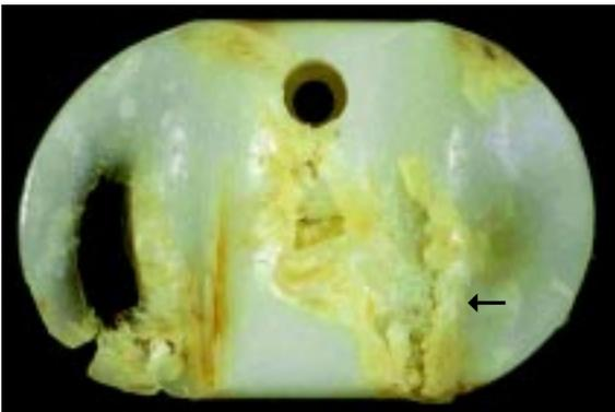
*Figure 7.6. Abrasion: a shredded or tufted appearance of the polyethylene (caused by direct contact with bone or PMMA).*
