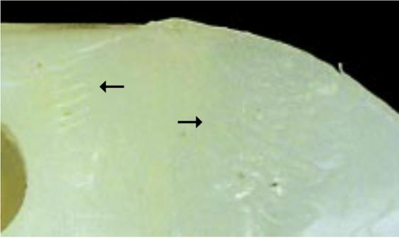
**Figure 7.19.** Screw marks were seen as striated impressions in the poly-ethylene (arrows).
