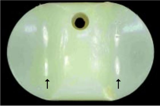
**Figure 7.1.** Burnishing. The medial and lateral sides of this retrieved PE insert have become highly polished.
