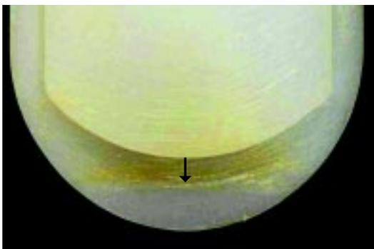
**Figure 7.23.** In 93.8% of the inserts that were available for analysis, surface deformation was seen at the edge of the tibial insert on the backside.
