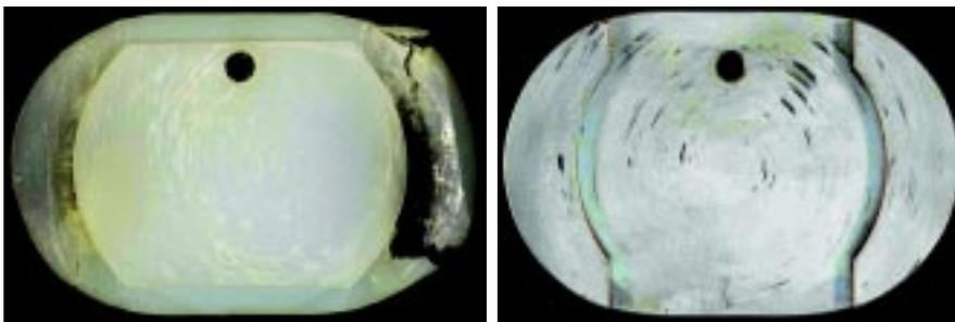
**Figure 7.22.** A rotational pattern of wear was seen on the backside of the polyethylene insert (left) and on the metal tibial tray (right). This pattern of wear was only seen in knees that had had loosening of the screw.
