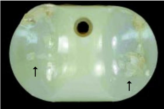
*Figure 7.5. Delamination: areas with evidence of a subsurface failure mechanism occurring parallel to the articulating surface.*
