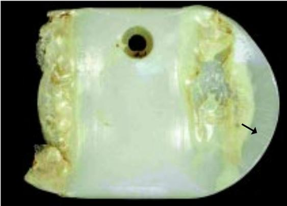
*Figure 7.4. Surface deformation: areas with permanent deformation occurring on or around the articulating surfaces, presumably caused by cold flow and /or creep.*
