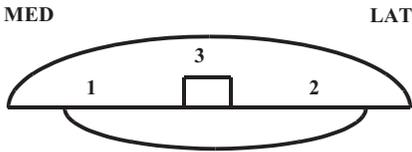
*Figure 6.5. Radiolucency zones 1 to 3 around the patellar component.*
